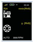
Detected speed value is displayed at the bottom. The word AUTO in front of the value informs, that automatic detection was used.
