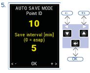
Select the time interval for data saving (1-60 minutes, 0 is for the maximum speed of data storage)
