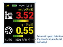
**RMS vibration values:** 10 - 1000 Hz in mm/s (ips) 0.5 - 16 kHz in g
