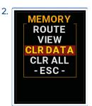
This removes all measured data. It removes route data and also the data saved manually (off-route). But the route structure (list of machines) is not removed and route can be collected again.
