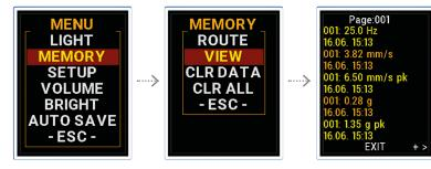
The list of saved readings appears. Every readings is described in two lines. The Point ID and value are on first line and time/date of reading on the second. Use Arrow buttons for listing.
