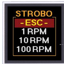
To adjust the tuning step, press the Enter button to get the Strobo menu
