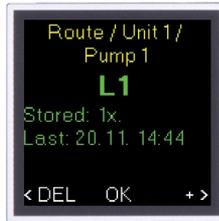
[DEL] delete the measurement [+>] save and move to the next point
