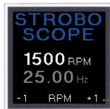
If the speed is found, the stroboscope frequency is set automatically
