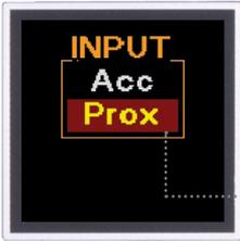
**i** The A4900 Vibrio MP needs to be connected to a proximity sensor for proximity measurement!
