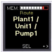
Use the Arrow buttons to switch between the machines in route
